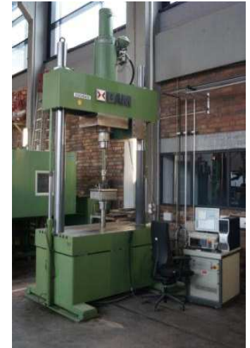
Test rig for small components (KPM), static and low frequency bedding modulus
