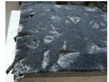
Ballast imprints on a USP sample
