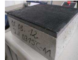
specimen, concrete block with USP
